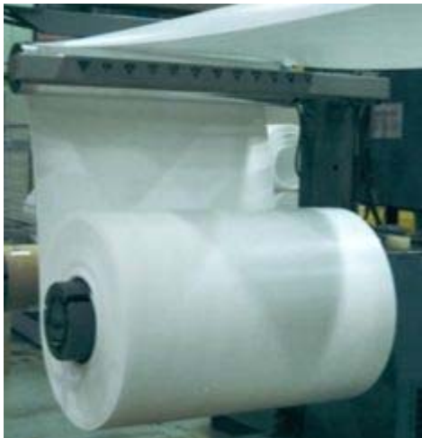
Ingeo foam made with Turbo-Screws technology (above & below)
